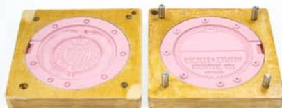
The molding box is now laid open showing the two halves of the silicon mold. Note the Robertson screw
