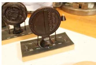
The wax patterns have been mounted on the base of the investment flask with the small vents installed on each side of the gating to allow for air escape when the metal is poured into the investment.
